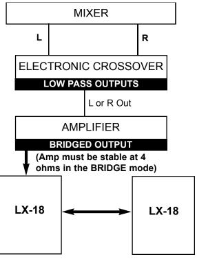
Connecting two LX-18 subwoofers in parallel results in a 4 ohm load.
